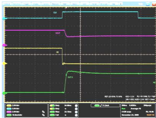
Figure 20: Turn ON output current characteristics (1)
